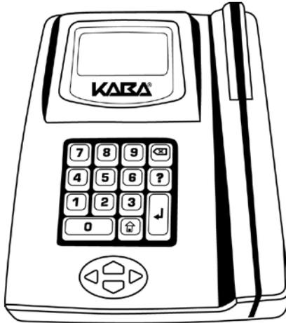
Full audit tracking capability is built into the FDU. Together with the lock audit trail, this information can determine which keycard was used to open a door and who issued that keycard.
